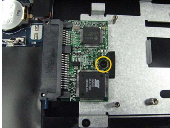
Figure 7 Removing the existing flash module
